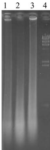
FIG. 1—One and one half percent agarose gel electrophoresis of DNA isolated from a cleaning trial of sheep femur. Lanes 1 – 3 contain 100 ng of DNA (based on OD readings) from bones cooked in water, bleach, and detergent/carbonate respectively. Lane 4 contains a size standard ( \lambda DNA digested with Hind III), in which the largest band is \sim 23 kb and the smallest is \sim 0.56 kb. Note the decreased amount of high molecular weight DNA in the bleach-processed sample, both in the gel and remaining in the well.
